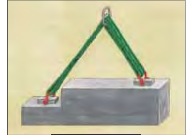
If the lifting points are an equal distance on either side of the center of gravity but one is higher, then the double sling should be attached to the higher lifting point.
