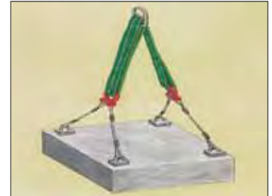
Never use the Twin-Path ® Adjustable Bridle in situations where the sling-to-hook angle is greater than 45°. Always connect above the center of gravity. If connections are made below the center of gravity, then the load may turn when lifted.
