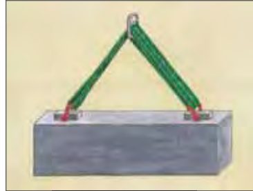
If the lifting points are an equal distance from the center of gravity then the Twin-Path ® Adjustable can be hooked-up with the double or single sling on either lifting point.
