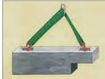
If one of the lifting points is closer to the center of gravity, then attach the double sling to this lifting point. It will have the highest weight concentration. If the Twin-Path ® Adjustable is attached so that the single sling is nearest the center of gravity, it will not allow the lift to be made.
